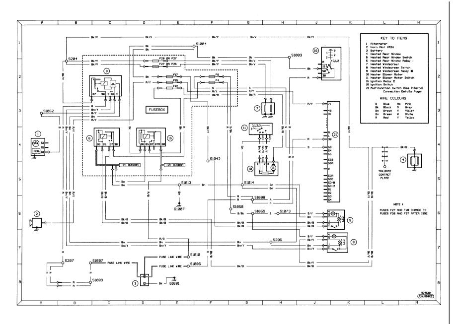
Diagram 3: Ancillary circuits - horn (except XR2i/RS models), heater blower and heated front /rear screens
